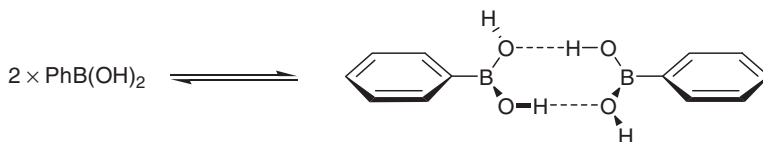
Scheme 8 Boronic acids exhibit a pre-disposition to associate as cyclic hydrogen bonded dimers upon crystallisation.
